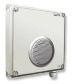
The VOX400 is a voice annunciator and MP3 player with built in amplifier and speaker. It can be triggered by using hard-wired alarm inputs, via RS485 or RJ45 Ethernet from other electronic equipment such as a computer or a DVR / NVR.
